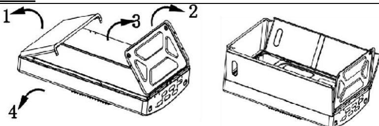
Disassemble the heater. Proceed in the order indicated by the arrows in the picture.
