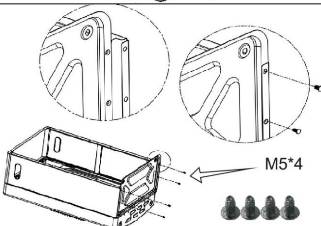
Secure the floor with 4 M5 size screws.
