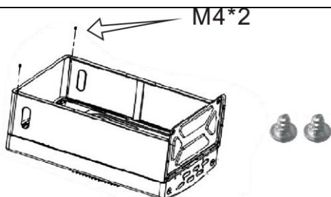
Secure the corner joints with 2 M4 size screws.
